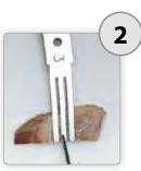
Cut other side of the central fork to obtain a pre-set thickness specimen.
