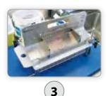
Slide side boards through grooves to hold specimen firmly in place
