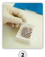
Place spacer on top of specimen
