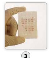
Close cover. Specimen will remain firmly in place during processing
