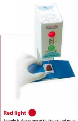
Sample is above preset thickness and must be re-cut or set aside for a more appropriate processing protocol.
