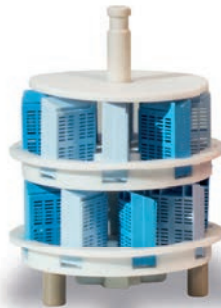
Mega - 16 cassettes For specimens 30x25x10 mm
