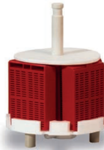
Super mega - 6 cassettes For specimens 70x50x15 mm
