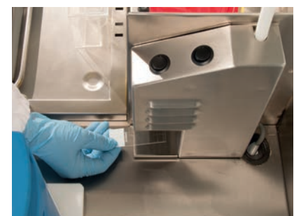
Forced air dryer for standardized drying of slides
